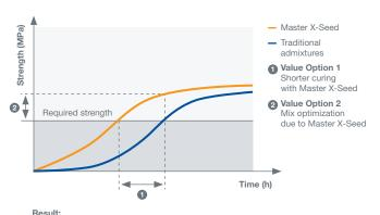
Result: Higher curing capacity due to shorter curing times or optimization of concrete mix
